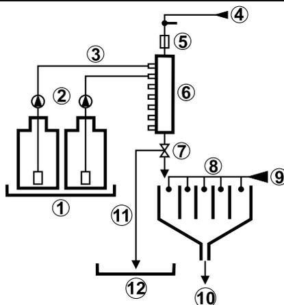
Multi-inlet dose controller with a compulsory rinsing device.
